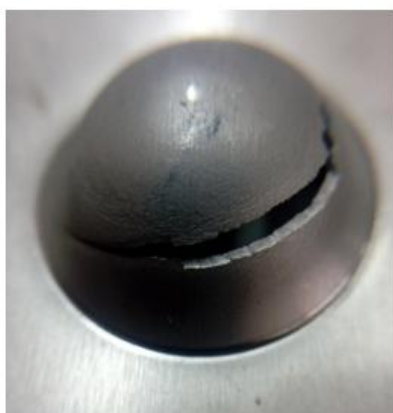
Figure 3 - View sample superalloy after the test Erichsen
